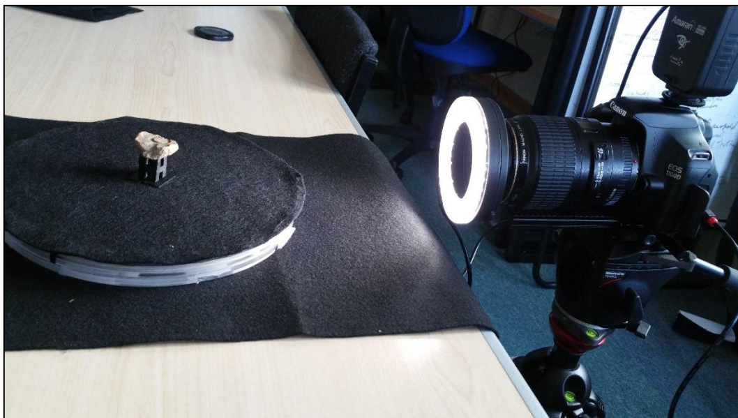
Figure 4 - Camera setup with light ring and mould fragment on custom made cradle.
