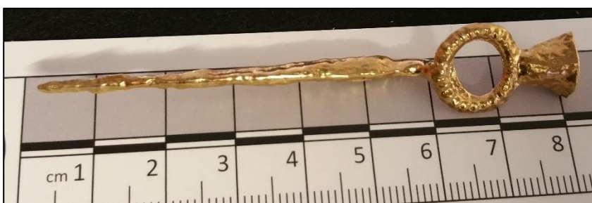
Figure 15 - 3D printed pin in bronze on cm scale.
